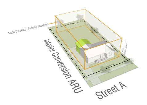
Type 1b. Interior Conversion in Your Existing Attached Garage to Create a new ARU
